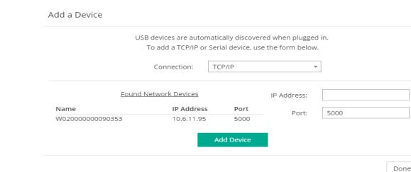
Select serial, and identify your serial port. Clicking the port select arrow should identify available comm's ports. Sensors are factory set to 115200 baud. Click Add Device, and Done:
