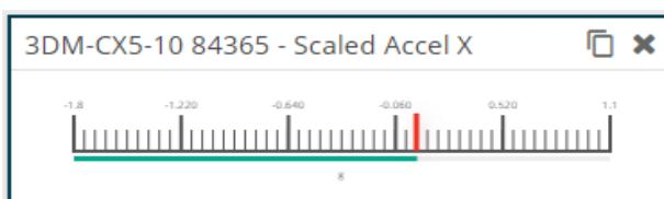
**Step 13:** If you click on the duplicate icon in this window, you can place two more linear gauges. Click on each of them, and select Accel, X and Y. You'll see the gauge displays move, as you manipulate the sensor.
