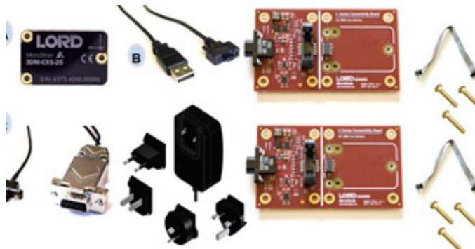
The sensor can be purchased by itself, or as part of a development kit. There are two variations of the kit. The 3DM-CX5-10 communicates via RS232, and is only supported by the RS232 version. (p/n 6212-3010). The kit includes the C-series Connectivity Board and appropriate cables and mounting screws. **This guide assumes that you have a development kit and will download the latest version of SensorConnect™ software.**
