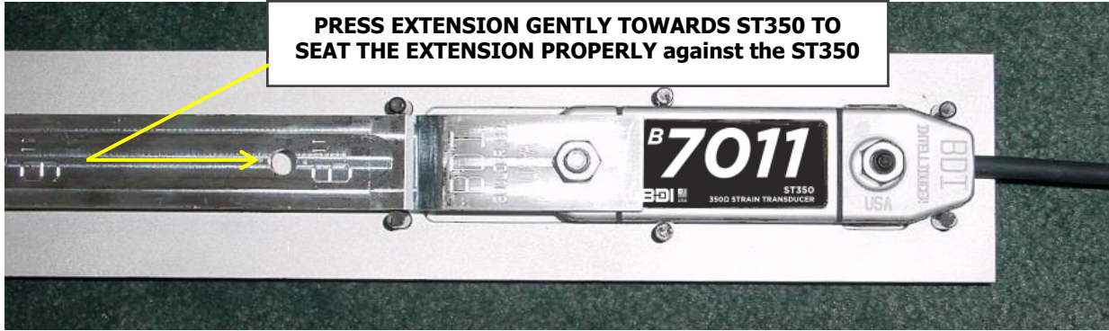
Figure 17: Aligning ST350 and Extension in the Jig
