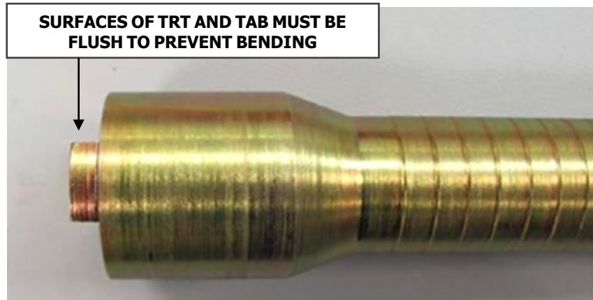
Figure 12: TRT with a Tab Inserted
