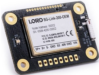
SG-Link ® -200-OEM - small, low-cost two-channel analog sensor node ready for OEM integration
