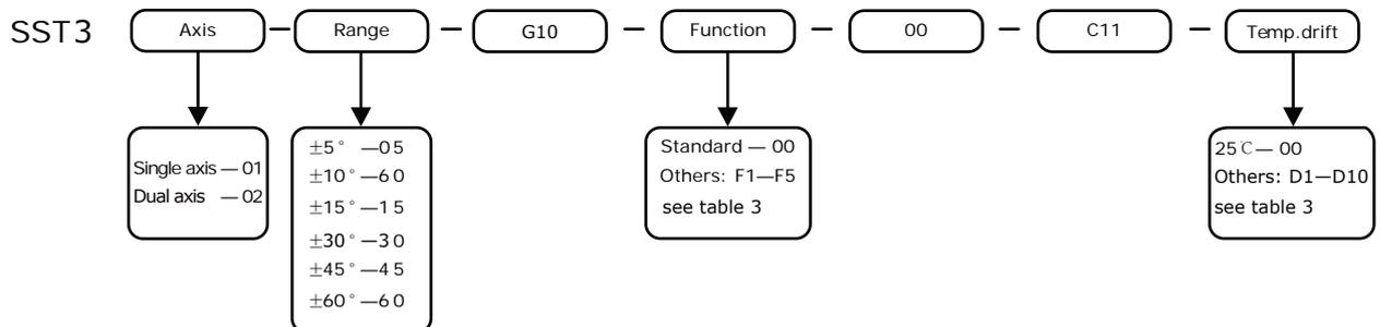
For example, if order a dual-axis USB inclinometer, with range  $\pm 15^\circ$ , the accuracy at room temperature is  $\pm 0.02^\circ$ , same the range of  $-20\sim 60^\circ\text{C}$ , USB output, 2m shield cable, anti-vibration module, the model should be SST302-15-G10-F5-00-C11-D3 (2m, enclosed referred disk (dynamic library, source code and instruction)
